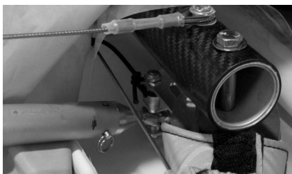
Figure 11 Washout Strut, Threaded Cone Connection
