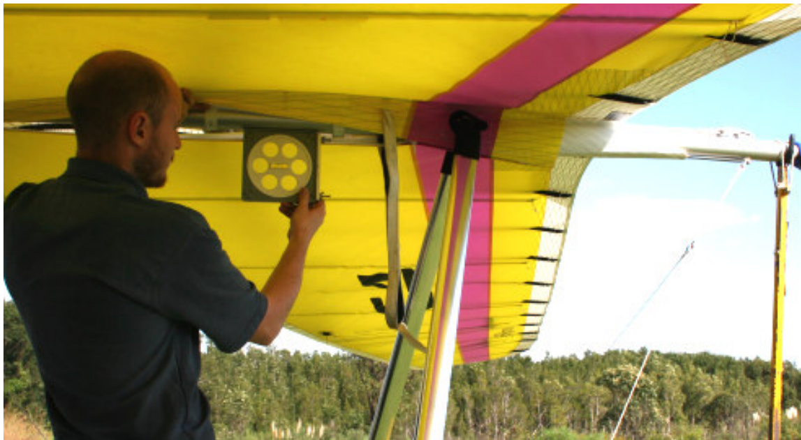
Figure 20 Setting Reference Keel Angle
