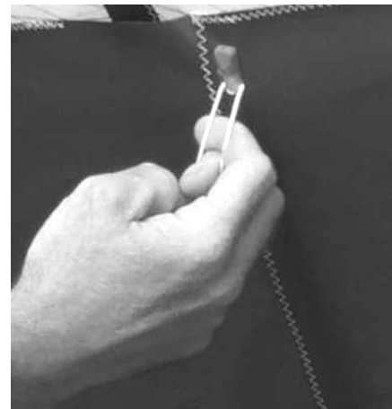
Figure 8 Insert Under Surface Battens
