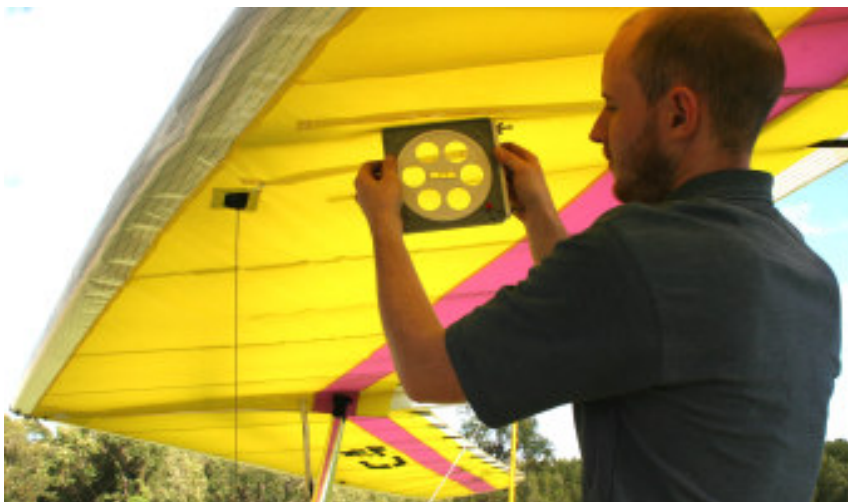
Figure 21 Measuring Washout Strut Angle
